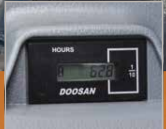
Hour meter (from ground level)
