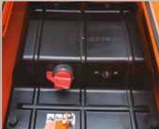
Battery cut-off switch
