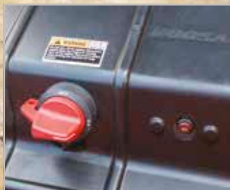
Battery cut-off switch
