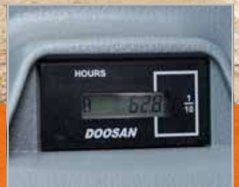
Hour meter (from ground level)
