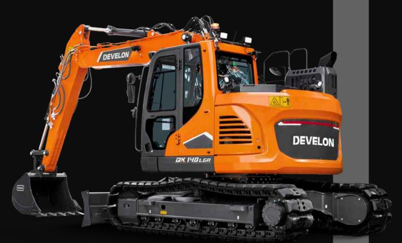
Maximum power115 hpOperating weight15.6 tBucket capacity0.51 m³
